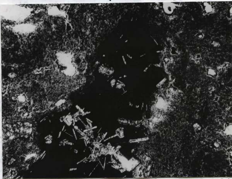
z.269. Glassy basalt xenolith, containing micro-phenocrysts of labradorite and prismatic augite, in the acid portion of the Upper Gilsardalur composite lava.
